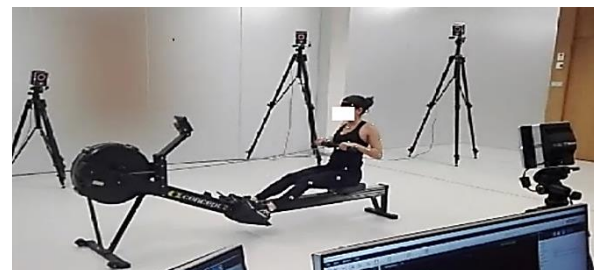
Figure 1. Status of the subject on the ergometer with motion cameras and indicators
