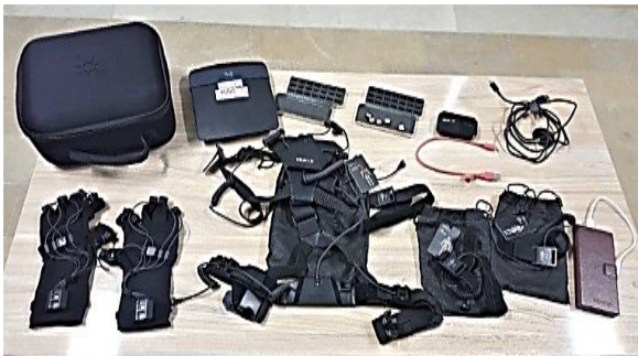
Figure 1. Items of the motion capture device, along with a power bank and a router used in the study
