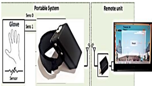
Figure 2. System designed to perform isometric neck exercises in the exergame group
